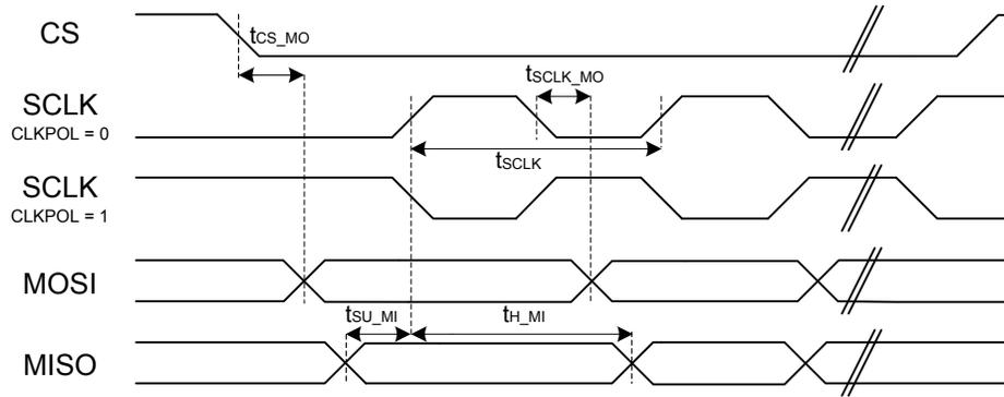
Figure 4.4. SPI Master Timing (SMSDELAY = 0)
