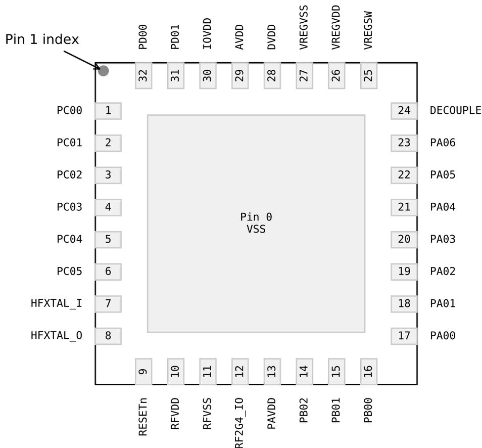
**Figure 6.3. TQFN32 Device Pinout**
