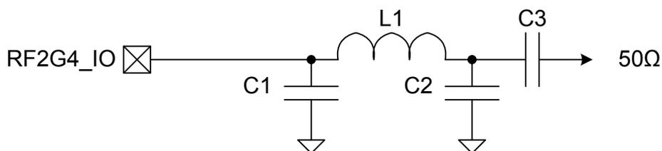
Figure 5.3. Typical RF impedance-matching network circuit
