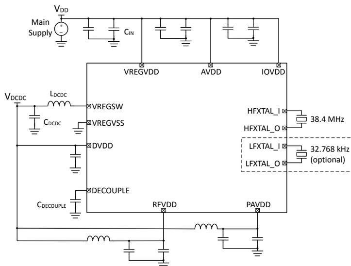
**Figure 5.2. EFR32BG22 Typical Application Circuit: DCDC Configuration**
