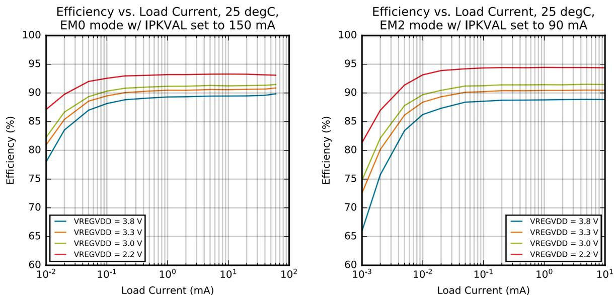
Figure 4.10. DC-DC Efficiency
