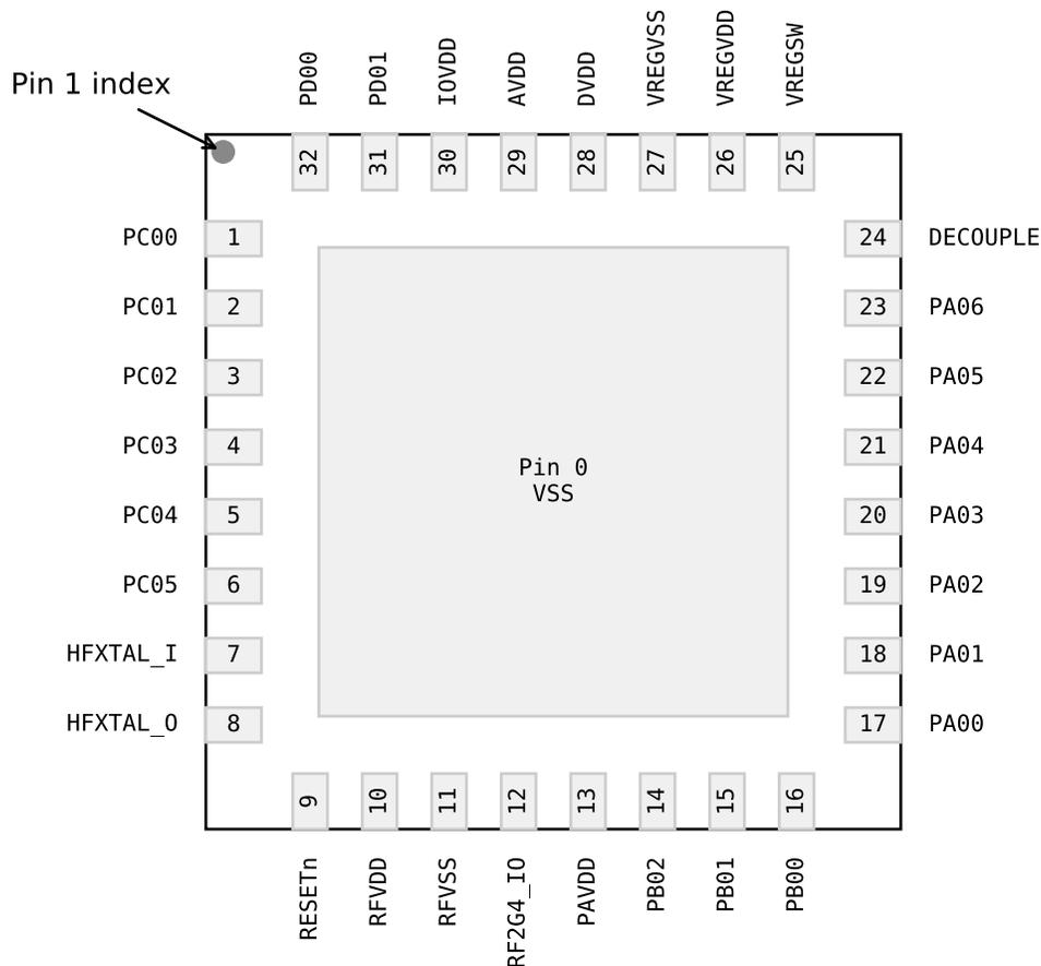
Figure 6.1. QFN32 Device Pinout
