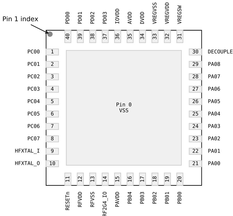
Figure 6.2. QFN40 Device Pinout
