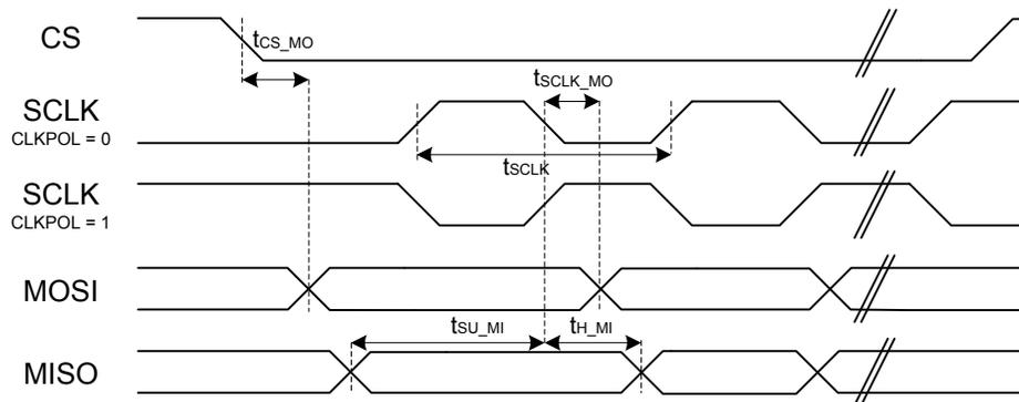
Figure 4.5. SPI Master Timing (SMSDELAY = 1)
