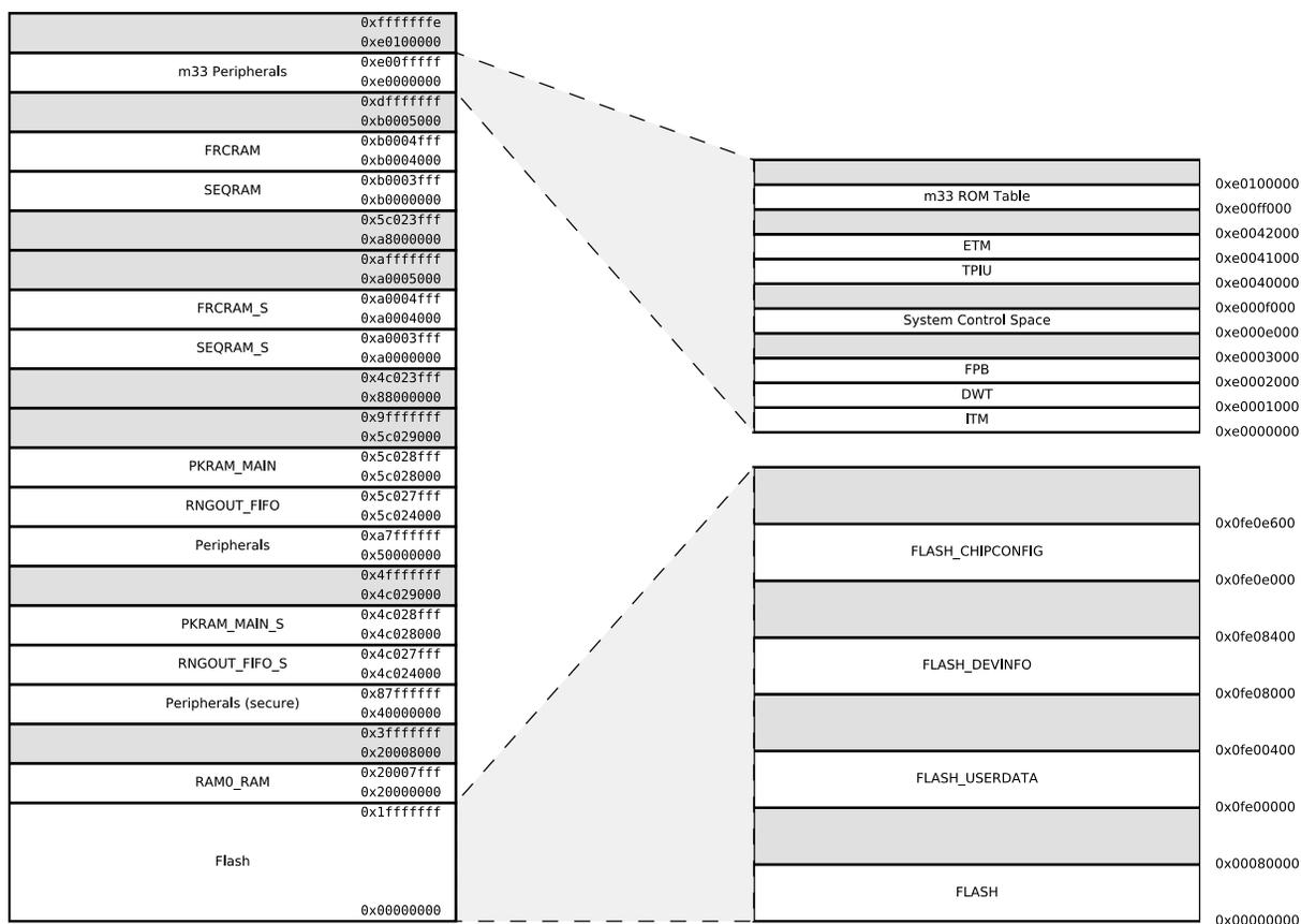
Figure 3.2. EFR32BG22 Memory Map — Core Peripherals and Code Space
