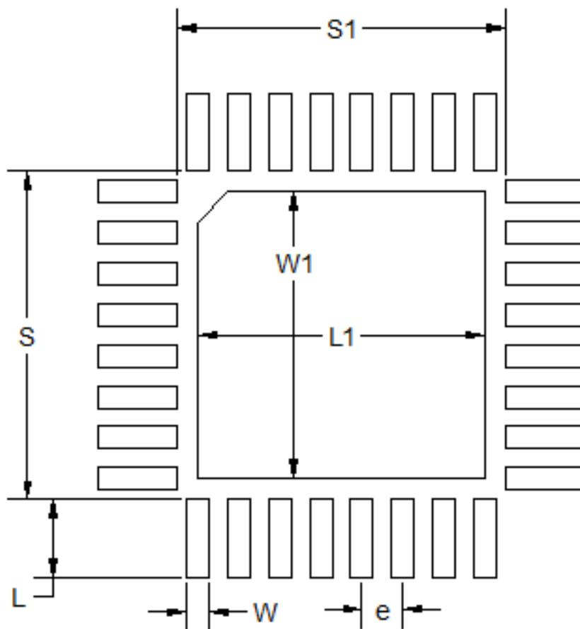
Figure 7.2. QFN32 PCB Land Pattern Drawing
