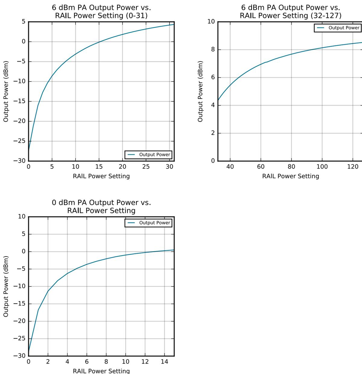
**Figure 4.9. Transmitter Output Power**
