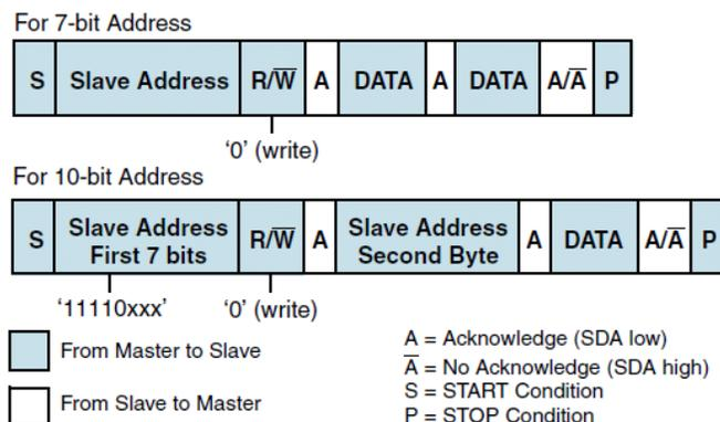
Figure 25: Master-Transmitter Protocol
