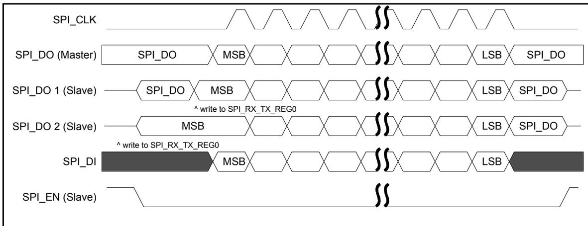
Figure 37: SPI Master/Slave, Mode 0: SPI\_POL=0 and SPI\_PHA=0
