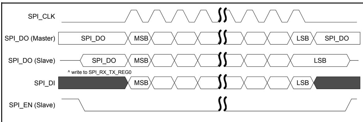
Figure 38: SPI Master/Slave, Mode 1: SPI\_POL=0 and SPI\_PHA=1
