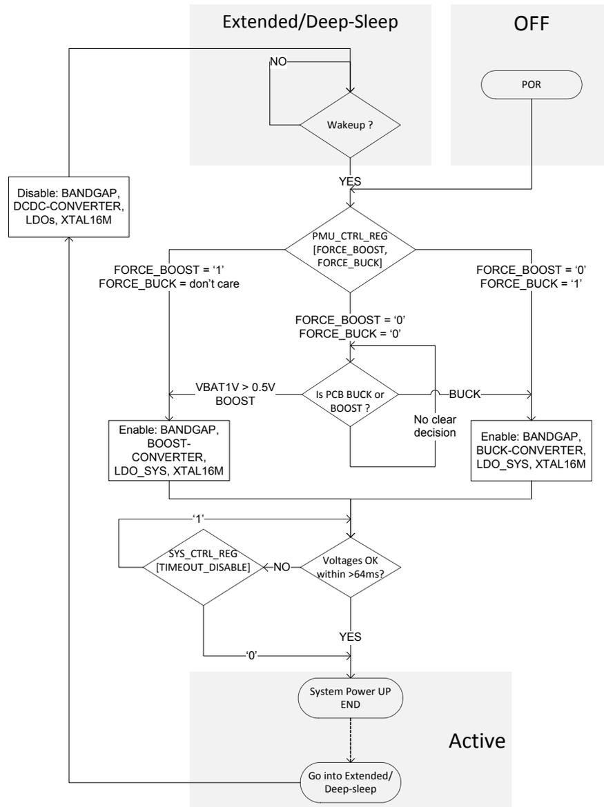
Figure 7: Power/Wake-Up Sequence
