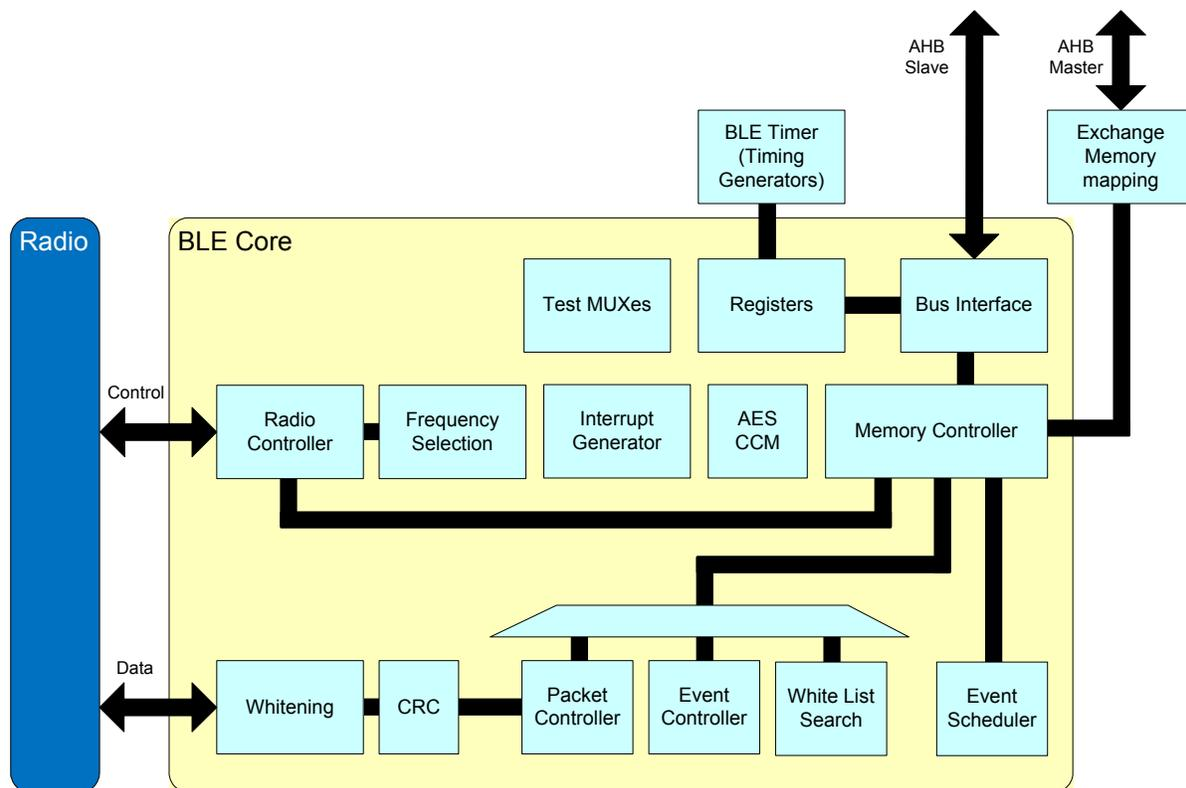
Figure 60: BLE Core Block Diagram
