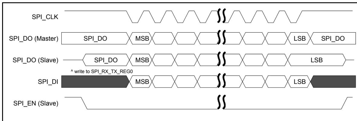
Figure 40: SPI Master/Slave, Mode 3: SPI\_POL=1 and SPI\_PHA=1
