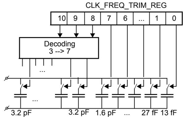
Figure 16: Frequency Trimming
