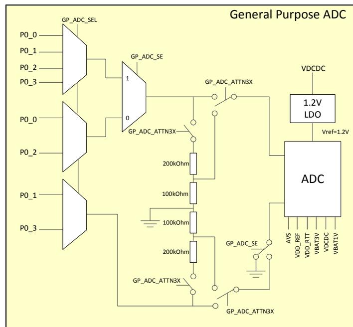
Figure 55: Block Diagram of the General Purpose ADC
