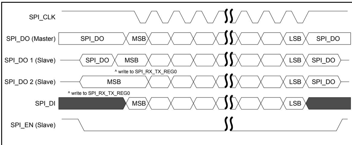
Figure 39: SPI Master/Slave, Mode 2: SPI\_POL=1 and SPI\_PHA=0
