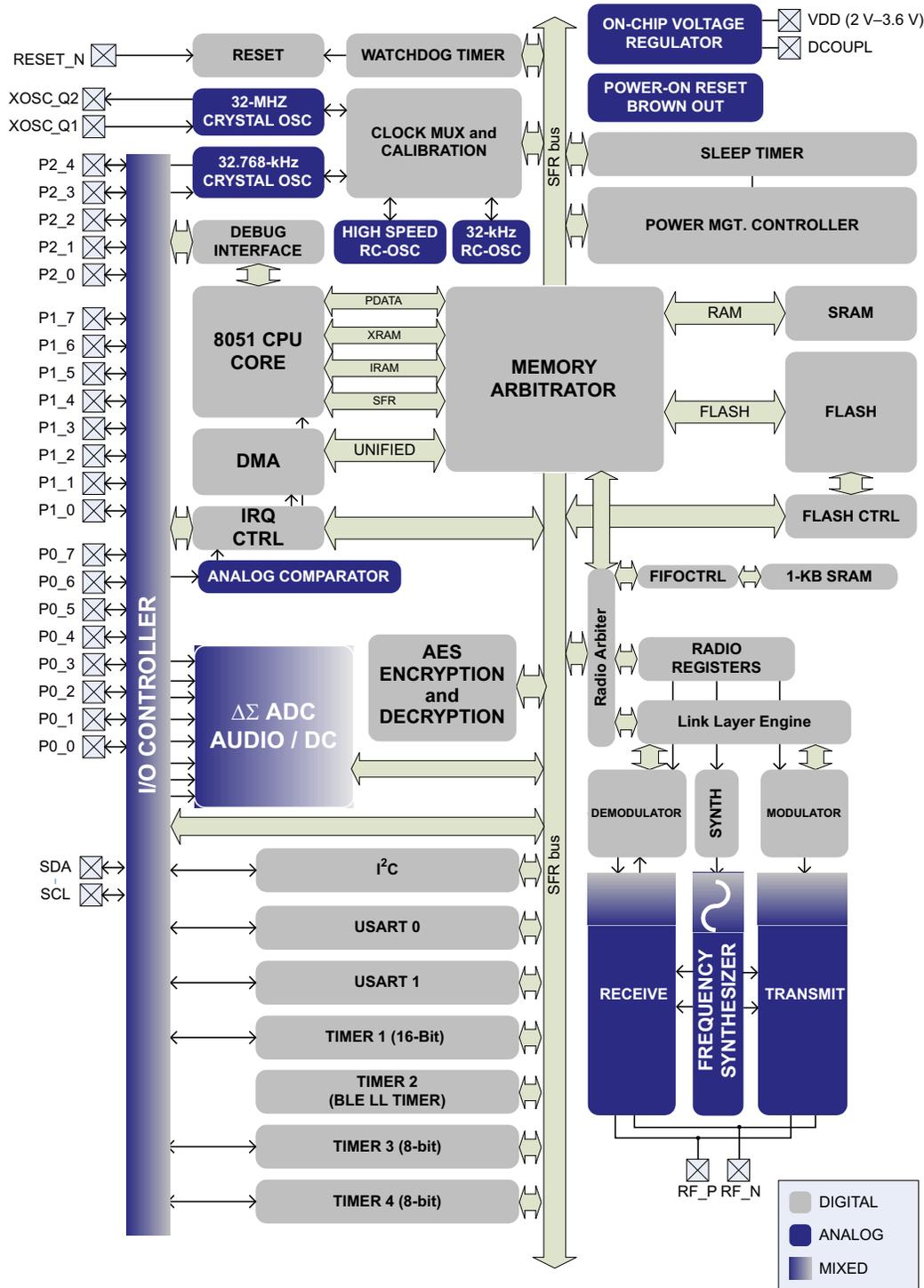
Figure 1. Block Diagram
