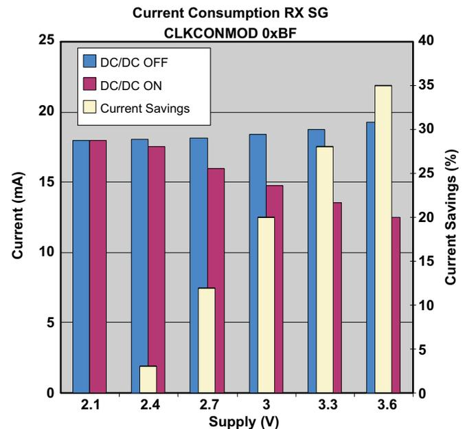
**Figure 21. Current Savings in RX at Room Temperature**
